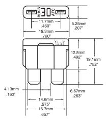
Catalog Symbol: ATC Fast-Acting Ampere Rating: 1 to 40 Amperes Interrupting Rating: 1,000 Amperes Agency Approvals: U.L. Recognized, (3-40A) Guide JFHR2, File E56412 Ordering: Specify packaging and product code
